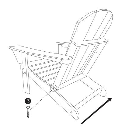
Connet part G (back cross-piece) to the seat panel using Hardware ③ (M6 x 40mm Screw). Secure part H (front cross-piece) to B (right leg) & C (left leg) using Hardware ③ (M6 x 40mm Screw). Congratulation! You finishes the assembly of this Adirondack Chair.
