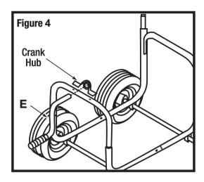
5. (SEE FIGURES) Attach the first hose reel (D) to the roller (I), on the end with the crank handle stem, using 6 bolts (5).
