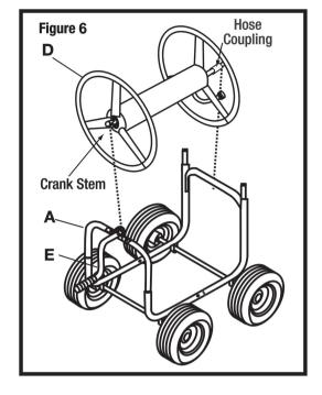
7. (SEE FIGURE 7) Insert bolt (3) through inside hole of crank stem and crank handle hole, Place flat washer (10) onto bolt (3) fasten with lock nut (11). Insert bolt (3) through outside hole of crank stem and crank handle hole and fasten with lock nut (11). Tighten all fasteners securely.
